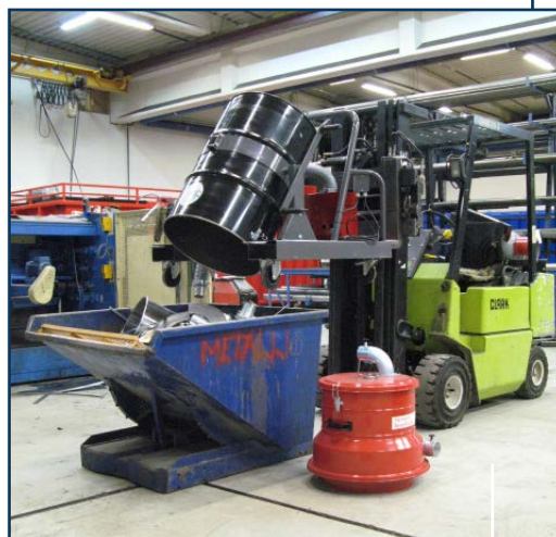
Crank emptying mechanism
