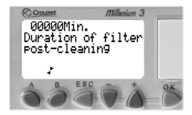
At this stage the total duration of the post-operation post-cleaning can be adjusted, the time is adjusted with the — and + -buttons and confirmed by pressing the OK button or by pressing the A button again, the following text will appear on the display:
