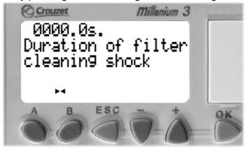
At this stage the compressed air pulse time of the filter cleaning can be adjusted, the time is adjusted with the — and  $\dotplus$  -buttons and confirmed by pressing the OK button **or** by pressing the **A** button again, the following text will appear on the display:
