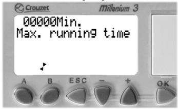
If you wish to disable the running time limitation, set the maximum time to 0min. In this case, the vacuum overrides the running time limitation and runs until the vacuum is switched off normally. The running time limitation has been disabled (0min) as a factory default.
