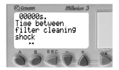
At this stage the pause time of the operation-term filter cleaning can be adjusted, the time is adjusted with the — and  $\dotplus$  -buttons and confirmed by pressing the OK button **or** by pressing the **A** button again, the following text will appear on the display:
