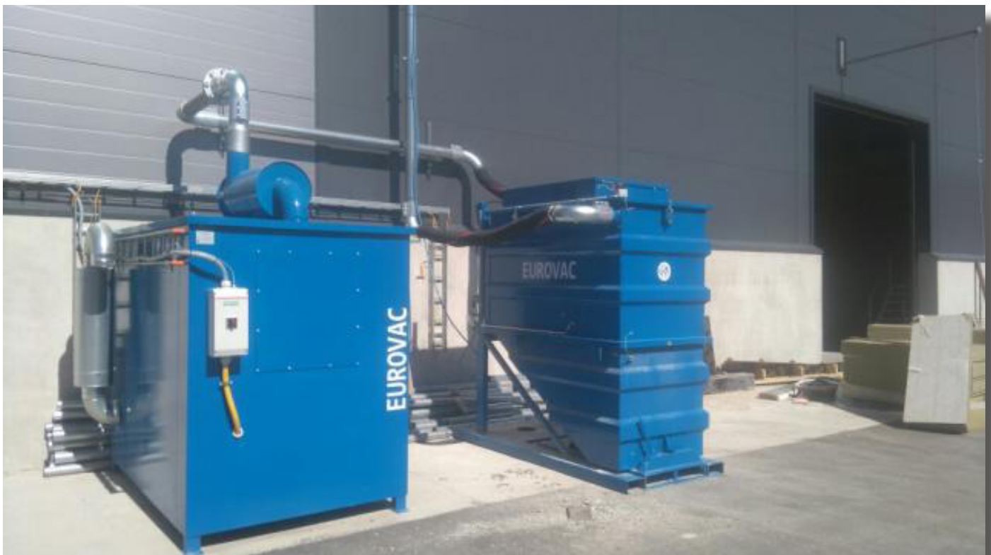
Eurovac 45 kW rotary piston suction unit + dump filtering unit
