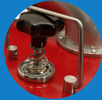
Filter cleaning with shaker rod
