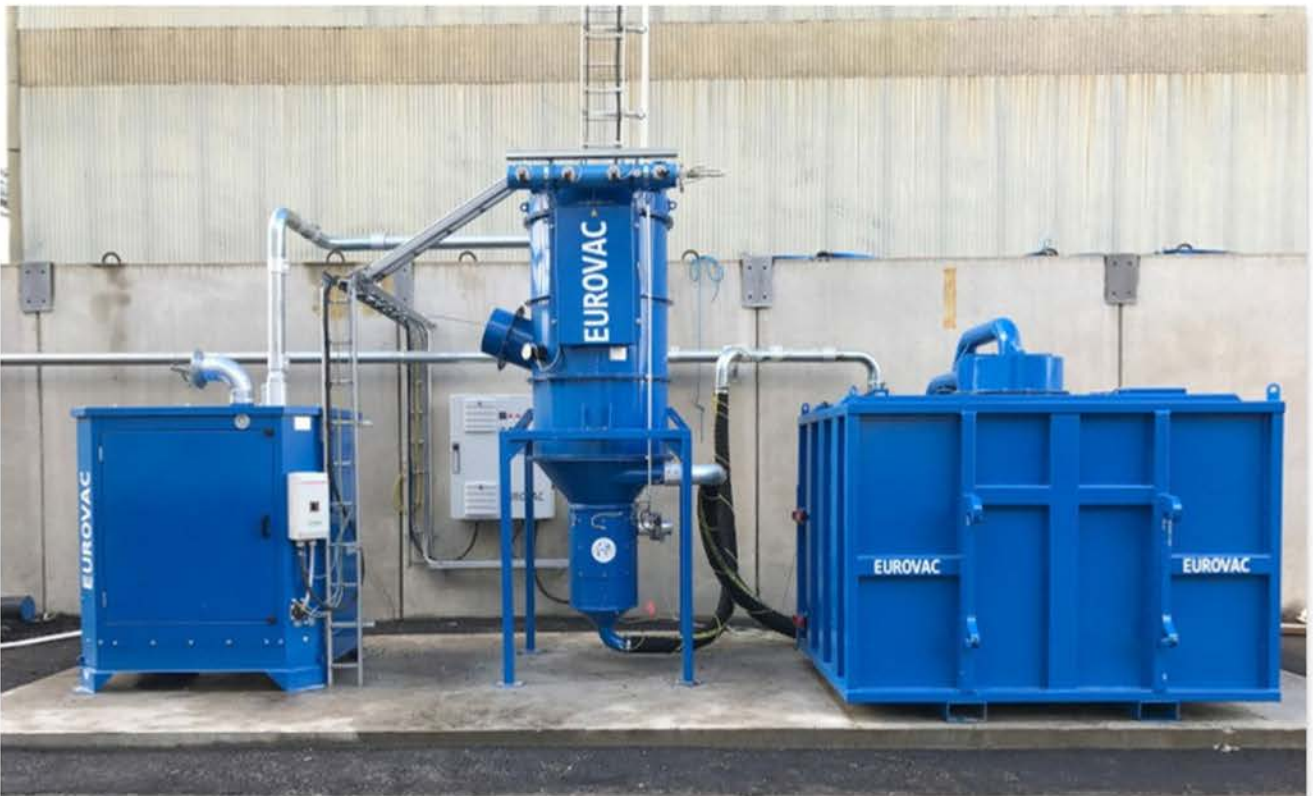
Eurovac 900 suction unit, 5 m 3 with pre-separator and 37 kW rotary piston suction unit
