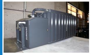
Roll off suction container with rotary blower 13m<sup>3</sup>
