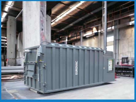
With a rotary blower, the dimensions of the roll off suction container  $13m^3$ : H 2530 mm W 2610 mm D 5950 mm Empty weight (45 kW) ~ 5300 kg
